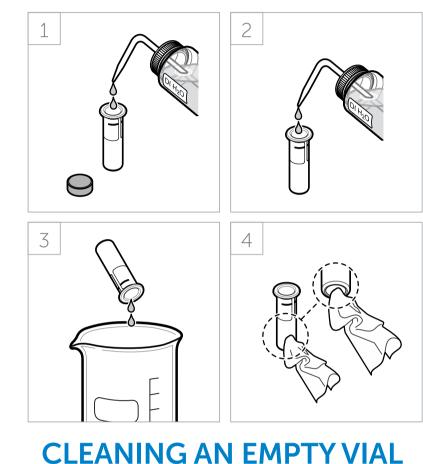
Make sure to clean the sides of the cells prior to measurements to remove fingerprints and other impurities.
