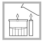
1. Blank: Transfer sample to a rectangular cuvette (50 mm or 10 mm).
