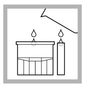
**6.** Transfer to a rectangular cuvette (50 mm or 10 mm).
