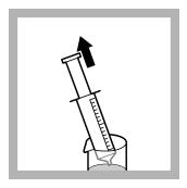
7. Draw about 10 mL of the sample which is to be filtered into the syringe.
