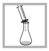
9. Filter the sample into a vessel provided for this purpose. The filtered sample can now be used for the required determination.
