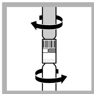
7. Tighten the cuvette combination again before inverting it.
