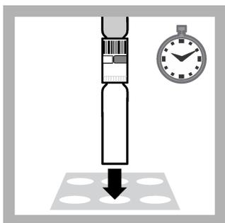
5. Heat in the thermostat (**blue indicator cuvette upwards**).
