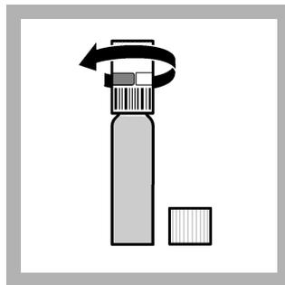
3. When the sample preparation is complete, open the blue indicator cuvette and **immediately** screw on the membrane double cap tightly. (The barcode label must point towards the indicator cuvette).
