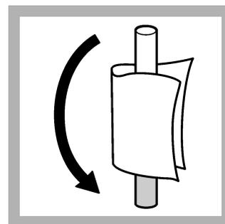
8. Invert cuvette combination, thoroughly clean the outside of the indicator cuvette and evaluate.
