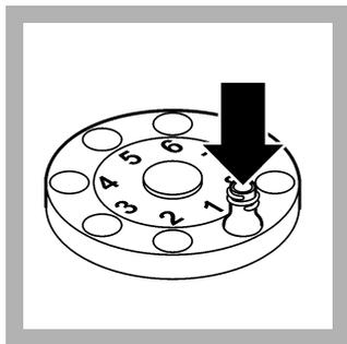
2. Insert the **open** digestion cuvette in the TOC-X5 shaker, pushing it down as far as possible. Position the fan cover over the cuvette. Switch on the instrument. After **5 minutes** an acoustic signal is emitted.
