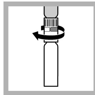
4. **Immediately** close the digestion cuvette tightly with the prepared indicator cuvette. Hold cuvette combination vertically. **Do not invert.**
