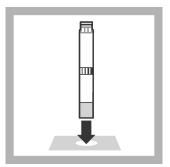
8. Insert the blank into the cell holder. In the pop-up window start the test Silver, total.
