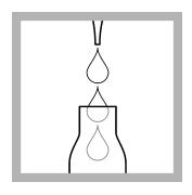
5. Carefully pipet into the Cuvette Test:1.5 mL of solution B.
