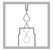
**1.** Add to a dry reaction tube: **10 mL** of **sample**.
